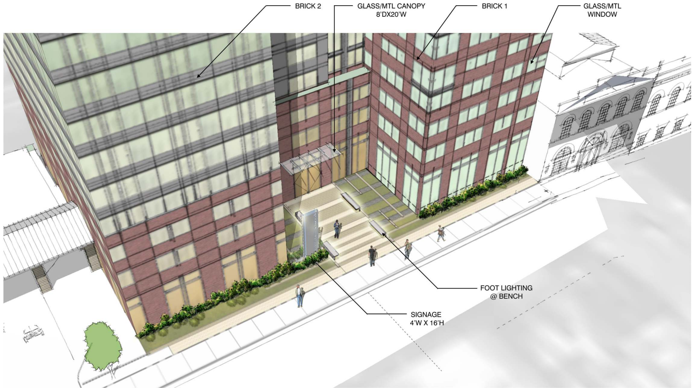
Figure 1-9: Entry Court Detail 1 Buena Vista Teutonia PUR City of Yonkers, Westchester County, New York Source: Lessard Design, 05/11/11
